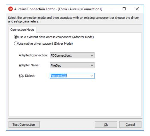
For that mode, choose an existing data-access component in the "Adapted Connection" combo. The dialog will list all the supported components. The component to be adapted must be placed in the same form or data module as TAureliusConnection. Components in other forms or data modules won't be displayed.
