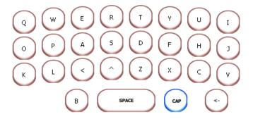
TMS touchscreen keyboard components offer TAdvTouchkeyboard & TAdvPopupTouchkeyboard. TAdvTouchkeyboard and TAdvPopupTouchkeyboard are components to display a configurable onscreen keyboard for touch screen applications. The keyboard has built-in settings for QWERTY, AZERTY, DVORAK, NUMERIC, CELLPHONE keyboards but also supports fully customizable keyboard layouts.
