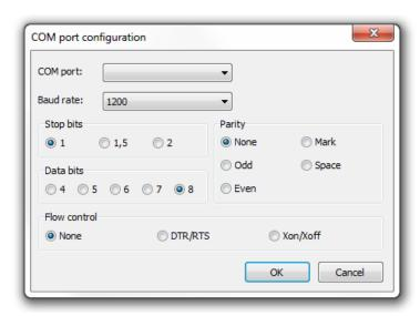
TVaConfigDialog will display the COM port settings as defined in the connected TVaComm component and after changing the settings via the dialog and closing the dialog with OK, the updated settings will be applied to TVaComm.
