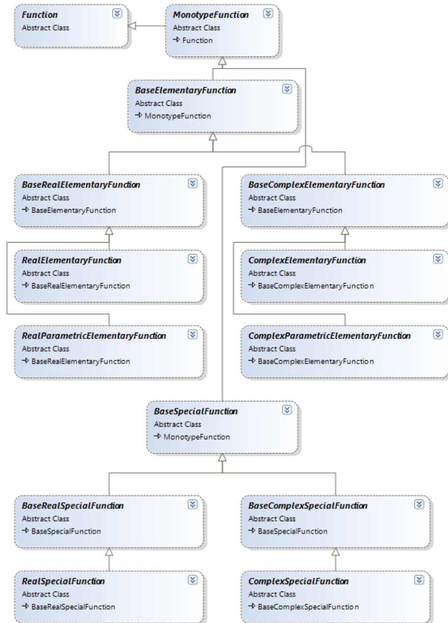
Picture 2.3. Function class hierarchy diagram.
