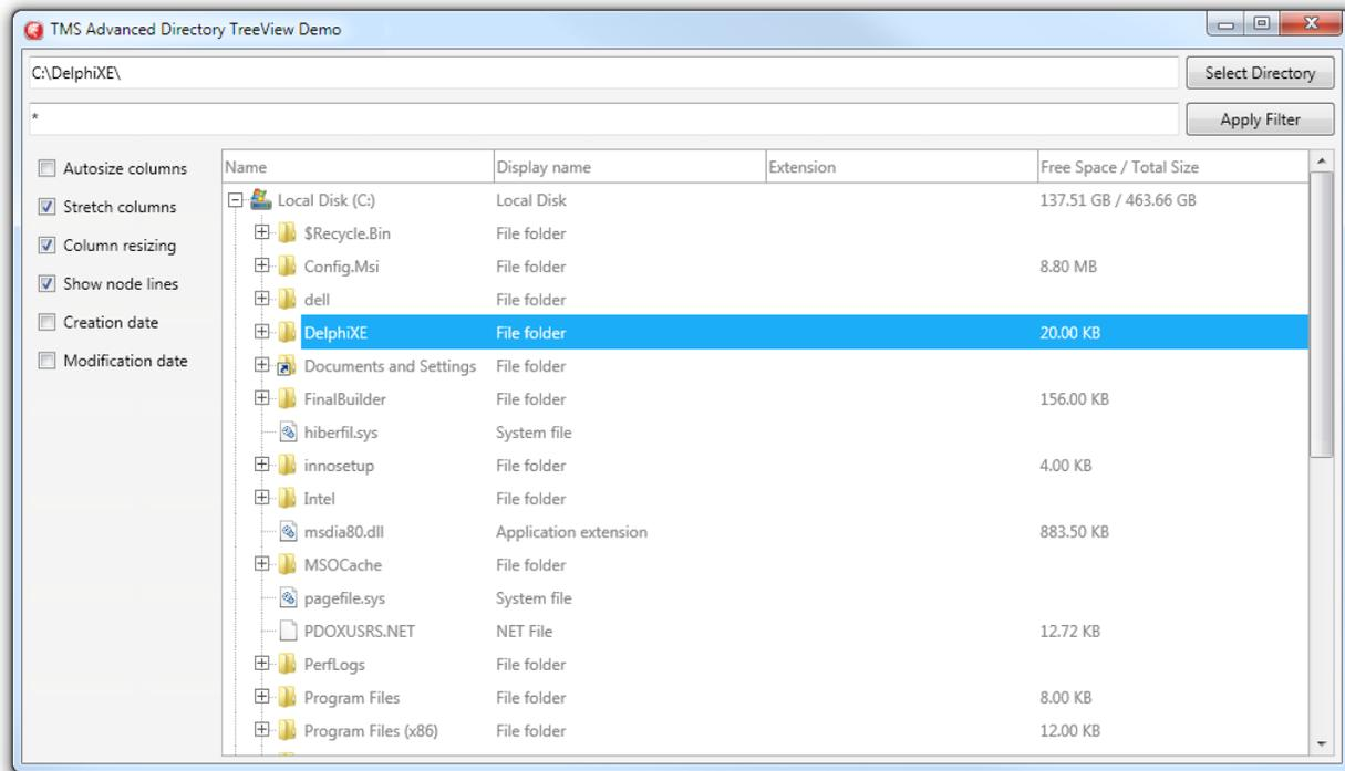
The Directory treeview demo uses the TAdvDirectoryTreeView component that is capable of loading a drive, or a folder and apply a filter. Additionally the column sizing, auto sizing of columns and stretching is demonstrated.
